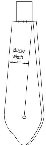
The auger bodies are manufactured in (non-toxic, not stainless steel) iron-manganese steel. The piston sampler is made of stainless steel. All auger bodies are unpainted for the purpose of environmental research.
