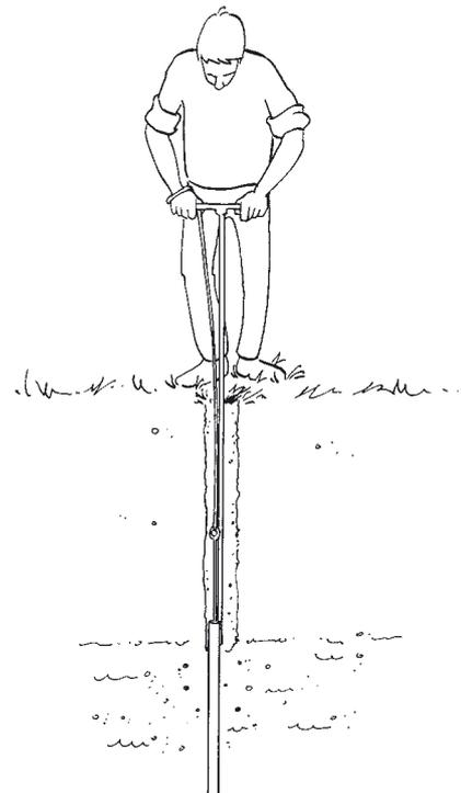
4. When the tube has been filled, push once more and pull it out of the auger hole.
