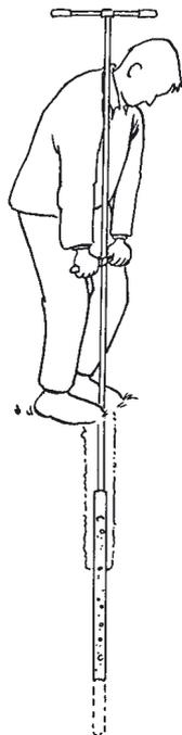
When augering at greater depth, attach extension rods to the upper end of the gouge auger, directly below the upper part. The rods tend to bend following the line of the auger hole. Follow the same order when (dis)connecting the rods.
