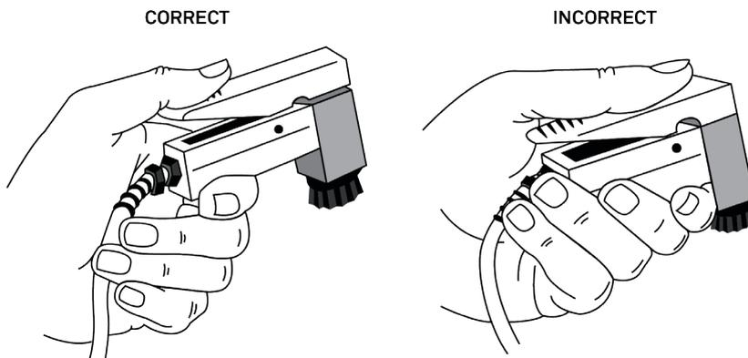
**Figure 4** Correct way to hold the sensor head
