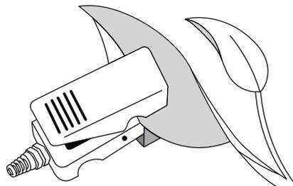
Figure 11 Leaf orientation during adaxial or abaxial conductance measurements
