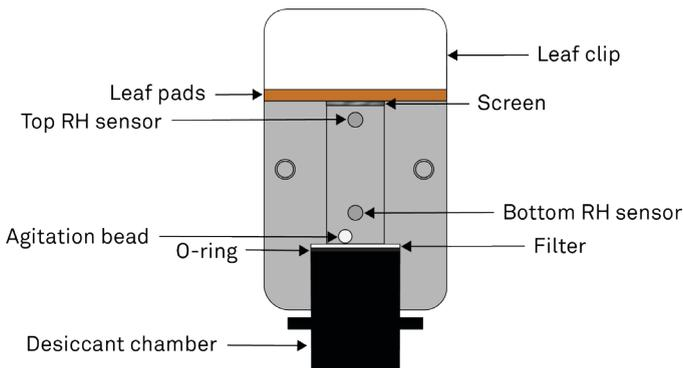
Figure 26 Sensor head internal components
