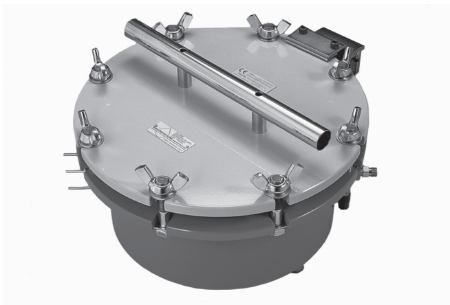
Fig. 5 1500F2 Extractor with lid attached
