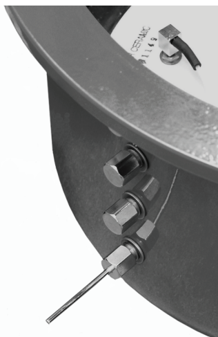
Fig. 10 - Fitting being screwed into the Outlet Port
