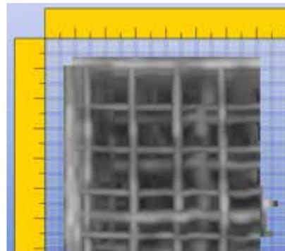
C-thru visualisation: dual antenna polarisation allows the optimal detection of both first and deeper levels of rebars
