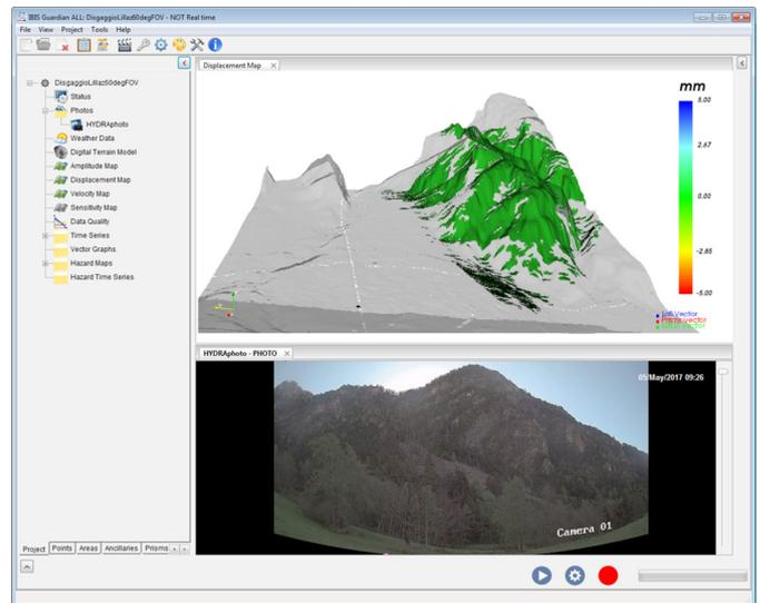
Cut-slope monitoring: displacement map and picture of the area
