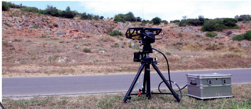
High-resolution radar system for early warning and real-time monitoring of buildings, dams, tunnels, mining infrastructures, and cut-slopes.
