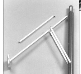
Big Hole Adaptor: An optional mechanical arm and pressure foot (shown here on the BHG-2) can be substituted for the spring to clamp the tool in large diameter boreholes. Conversion is easily done by the user in minutes. Multiple arms provide for various diameter holes. Largest arm extends diameter up to 480 mm (19 inches). When retracted, will fit inside a 75-mm (3-inch) diameter borehole.
