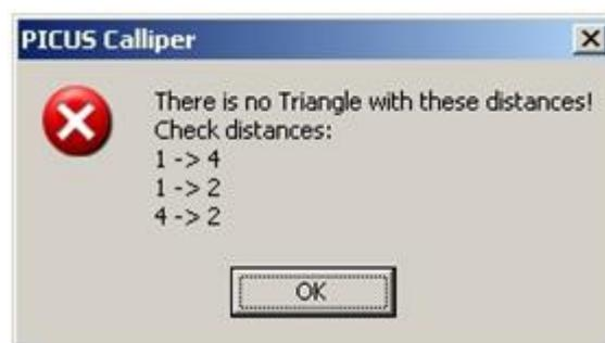
This message tells us that the program is unable to calculate a triangle using the distances measured (in this case a triangle with points 1, 2 and 4). While working with the calliper in this situation you should keep an eye on the PC screen.
